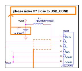
Figure-2: PL-2303H and PL-2303HXD Schematic Diagram (5V Capacitor) Comparison
