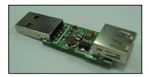
Figure-3: USB 5V-to-6.5V Port Converter
